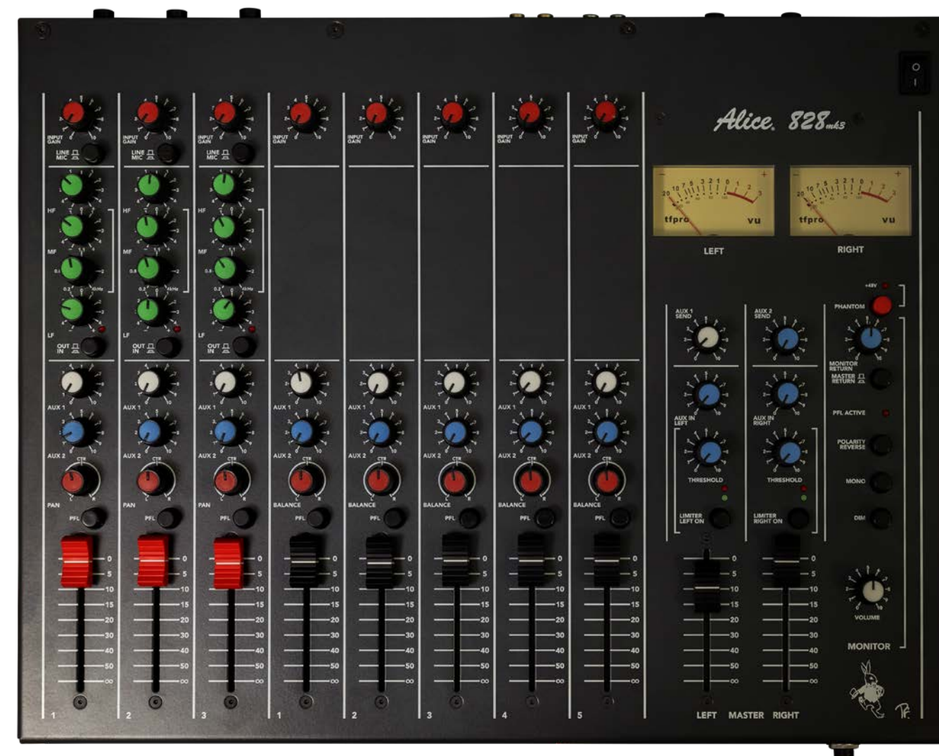
The standard configuration has three mono and five stereo input channels. Only the mono ones have mic amps and EQ, though Alice say that as the desks are hand-made at their factory, all manner of user-customisations, including stereo channel EQs, can be specified when ordering.
