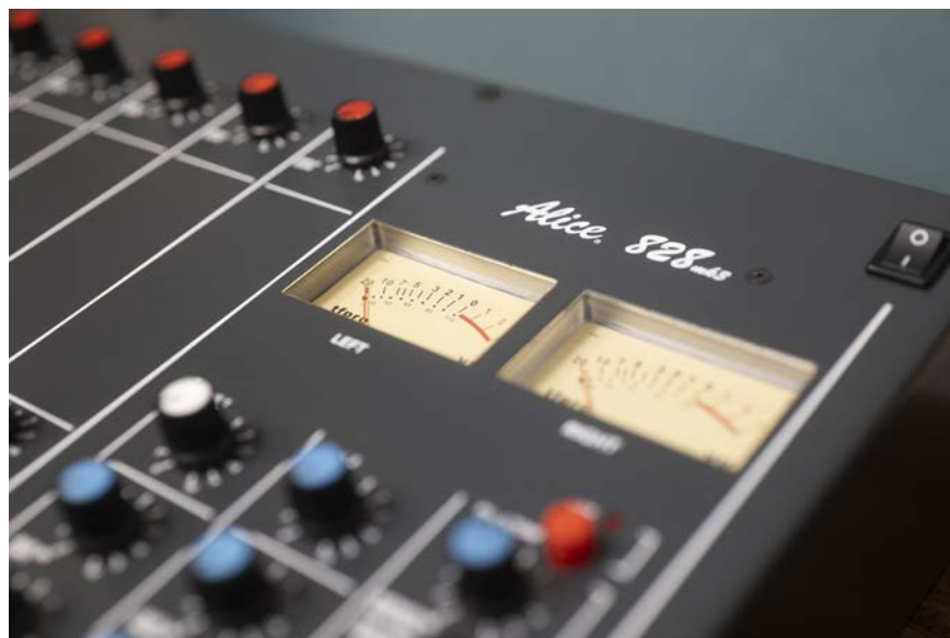
■ The two master-bus VU meters are the only visual indication of level on the desk — though that's not necessarily a bad thing if you're looking to drive the circuitry into saturation!
